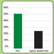
Use of a permanent split capacitor design allows the motor to deliver more power, while producing less waste heat than a shaded pole design.
